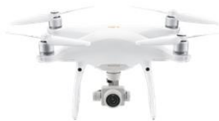
Photograph 1. Phantom 4 Pro Quadcopter from DJI
