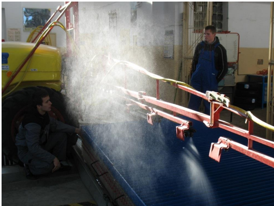
Figure 6.3. Threats for operators doing tests of distribution of nozzle liquid fall on the groove table
