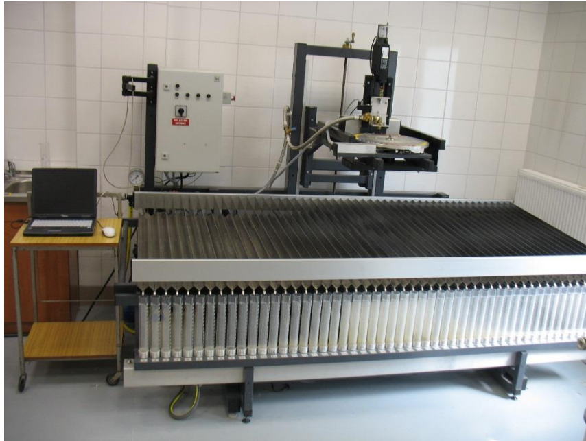
Figure 6.4. Device testing to investigations of crevice agricultural nozzles
