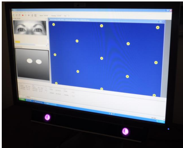
Figure 5. Calibration of a SensoMotoric Instruments (SMI) eye tracker Source: author's own materials.
